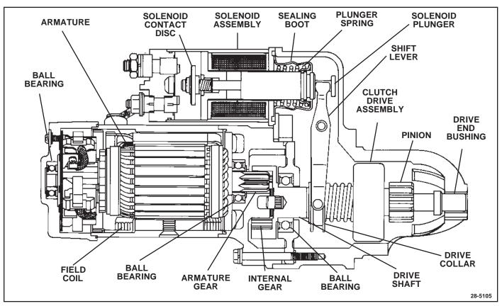
**Figure 2. Starter Cross Section**
