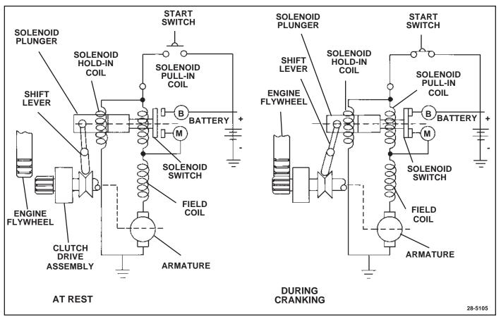
Figure 3. Starter Electrical Schematic
