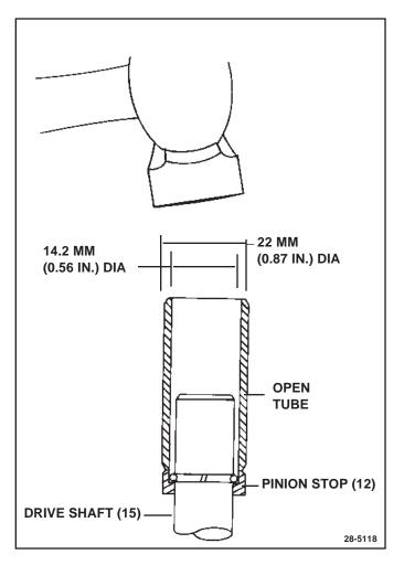
Figure 11. Removing Pinion Stop
