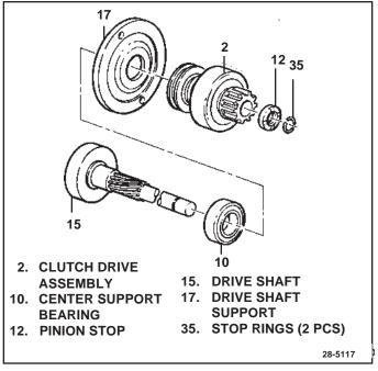
Figure 10. Drive Shaft and Clutch Group
