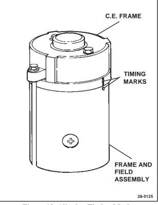
**Figure 18. Aligning Timing Marks**
