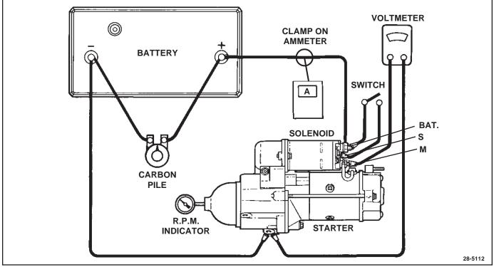
Figure 5. Starter No-Load Test Hook-Up
