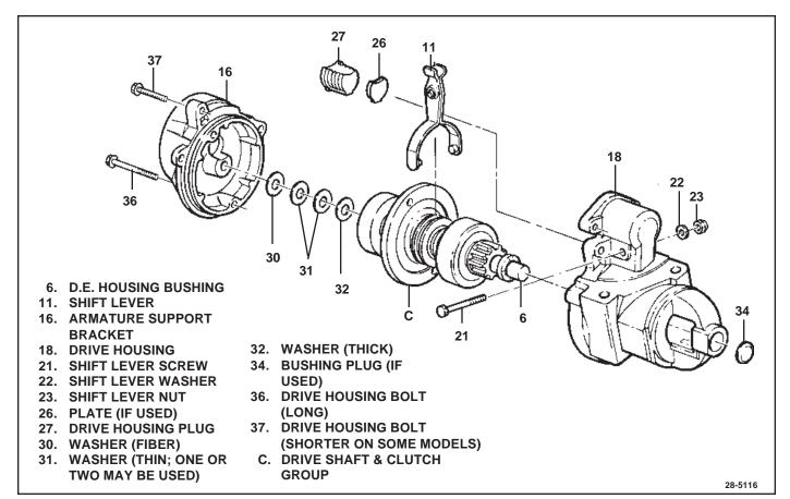
Figure 9. Gear Reduction and Drive Group
