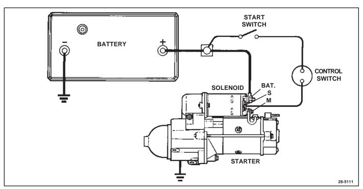
Figure 4. Starter Wiring Circuit
