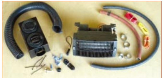
Here you see the Mojave Heater, the factory Defroster Plenum, and all the other parts needed for the install.
