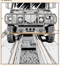
**6.** Rotate the tires by moving the vehicle straight forward until the center points of the two + marks are 16 1/2 inches above the ground at the rear side of the tires.
