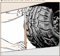
7. Measure the distance between the center points of the two + marks again and write it down.
