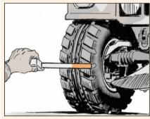
**5.** Measure the distance between the center points of the two + marks and write it down.
