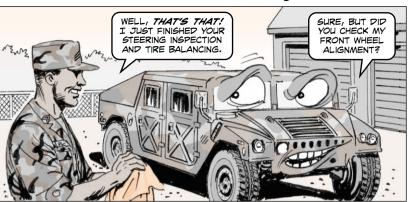
All the steering inspections and tire balancing in the world won't do much good unless you mechanics make sure the front wheels are properly aligned.
