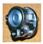
Inspect the new pump to make certain it is the proper one for your application. Although all P-type pumps look very similar, there are distinct differences. All 1980 and newer Saginaw equipped vehicles were equipped with metric pumps and an o-ring type pressure fitting. 1979 and earlier vehicles were equipped with SAE pumps containing a flare type fitting.
