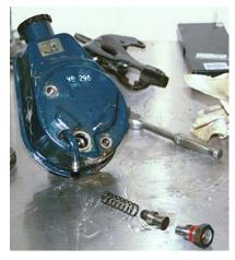
**Step 6** Grip the pump by its drive shaft and surrounding case, then use a soft-faced mallet and tap around the edge of the tin reservoir to remove it from the pump.
