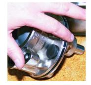
**Step 3** Install the lathe cut o-rings on the back side of the pump in the recessed areas around the threaded bolt holes and the pressure line port.
