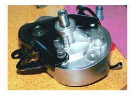
Step 9 Install the pump pulley onto the pump. Always use a pump pulley installer to push the pulley back onto the pump drive shaft. The hub of the pulley should be flush with the end of the drive shaft.
